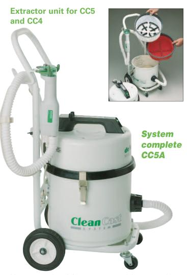
The four stage filtration system consisting of an easy to change disposable collection bag, two cloth filters and a micro filter. The micro filter retains 99.997% of all dust particles greater than 0.5 microns.
